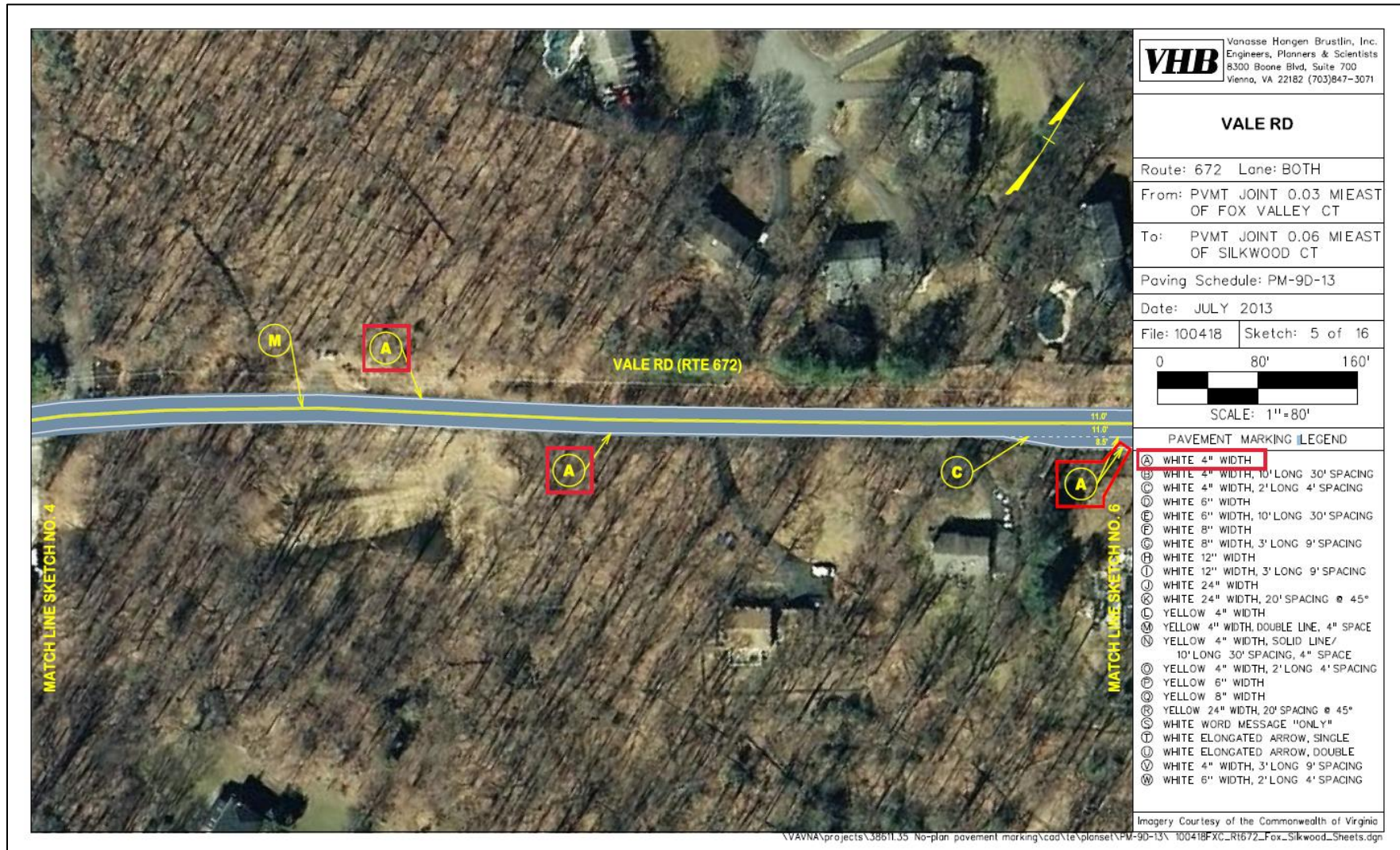
Figure 2: Example Design - Regular Width Edge Line Markings (Plan Sheet)
