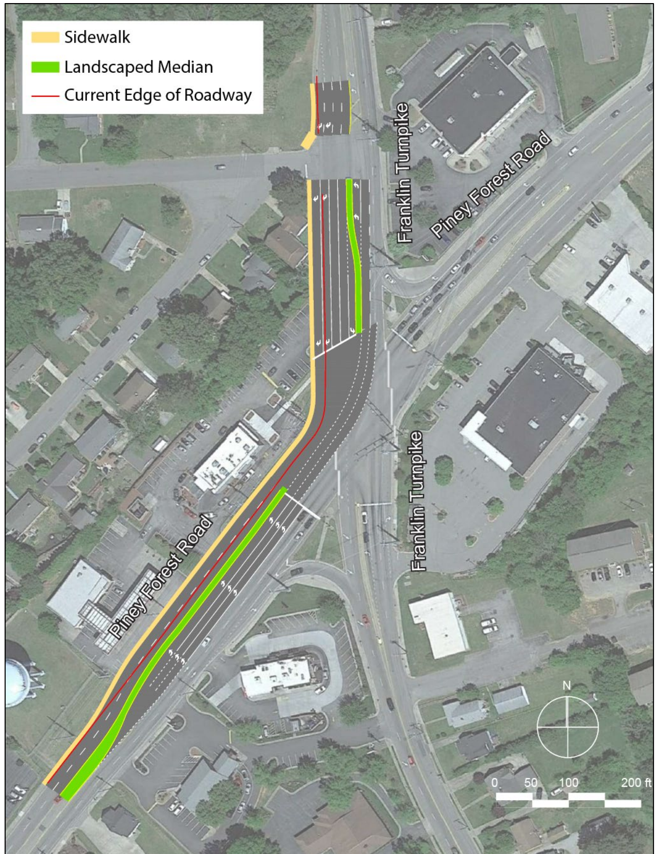
FIGURE 47: FRANKLIN TURNPIKE NORTHBOUND TRIPLE LEFT TURN LANES
