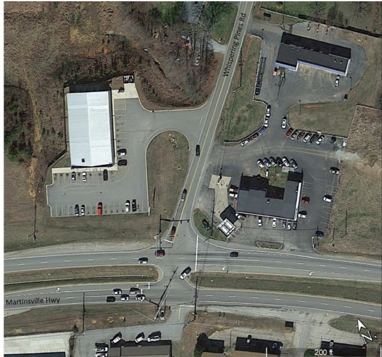
FIGURE 35: ENTRANCE SPACING AT WHISPERING PINES ROAD. ENTRANCES TO THE CHAMPION GAS STATION DO NOT MEET VDOT SPACING STANDARDS.
