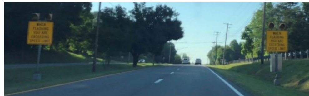
FIGURE 17: SPEED WARNING SIGNS ON RIVERSIDE DRIVE APPROACHING BARRETT ROAD.
