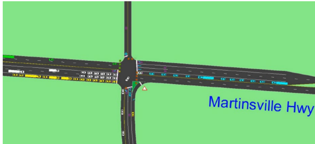
FIGURE 21: BERRY HILL ROAD INTERSECTION IMPROVEMENT PROJECT SKETCH. THIS SYNCHRO SCREENSHOT SHOWS THE NEW NORTHBOUND APPROACH CONFIGURATION AND EXTENDED EASTBOUND TURN LANES.
