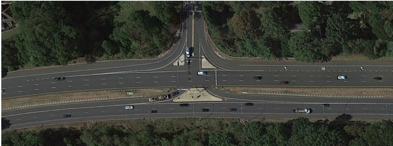
FIGURE 59: CONTINUOUS GREEN T INTERSECTION. A CONTINUOUS GREEN T IS USUALLY IMPLEMENTED ON THREE LEG INTERSECTIONS AND FORMALIZES A TWO-STAGE LEFT TURN MANEUVER FROM THE SIDE-STREET. IT CAN BE IMPLEMENTED AS A SIGNALIZED OR UNSIGNALIZED INTERSECTION. THE PROJECT TEAM TESTED AN UNSIGNALIZED CONTINUOUS GREEN T CONFIGURATION FOR THE SOUTHBOUND APPROACH OF STONY MILL ROAD WITH AN ADDED RIGHT-IN/RIGHT-OUT ONLY CONFIGURATION FOR THE NORTHBOUND APPROACH.
